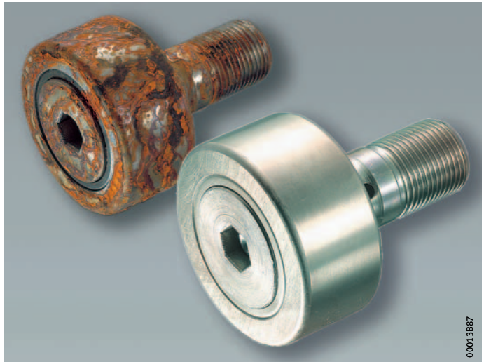
Figure 1 Track roller without and with Corrotect A* coating after salt spray test
